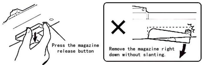
1. Press the magazine release button to remove the magazine.
