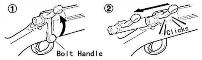
2. Return the bolt handle and put down ( If the bolt handle is not put down completely, you can not pull the trigger ).
